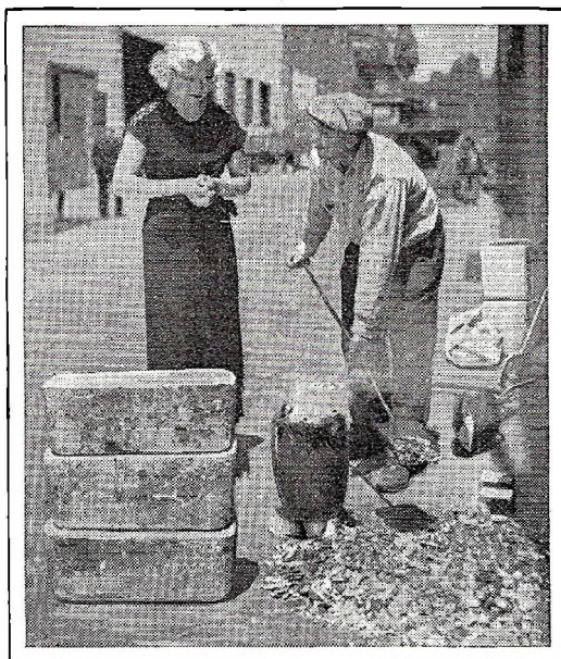
Flakes of silver in pile on street were recovered from old film developing solution by new electrolytic process. After melting, they are cast into 60-lb. bars shown at left of crucible.
