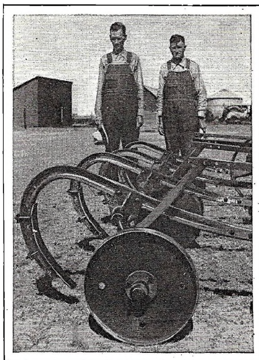
Photo shows the deep-furrow plow built by R. B. Duckett, Oklahoma farmer-inventor. Note how narrow steel plow blades are attached to, and fit the curve of the lister beam.
