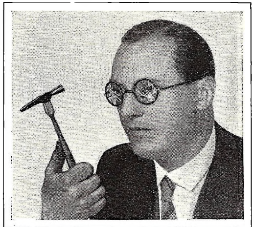
Photo shows the shatter-proof spectacles with glass intact. Subject holds the tool with which the glass was tested.
